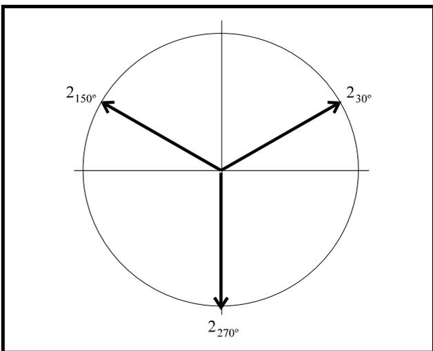
$$\begin{cases} k=0 \Rightarrow \alpha_1 = \frac{90^\circ}{3} = 30^\circ \\ k=1 \Rightarrow \alpha_2 = 30^\circ + 120^\circ = 150^\circ \\ k=2 \Rightarrow \alpha_3 = 150^\circ + 120^\circ = 270^\circ \end{cases}$$
